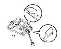
(b) Using a screwdriver wrapped with protective tape, disengage the 2 claws and 2 guides, and remove the 2 No. 1 room light covers.
