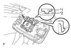
(a) Align the switch parts shown in the illustration and engage the 4 claws to install the room light switch base to the No. 1 room light assembly.
