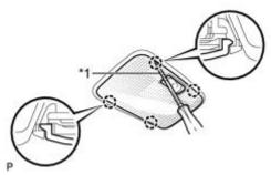
(a) Using a screwdriver wrapped with protective tape, disengage the 4 claws and remove the No. 1 room light lens.
