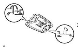
(b) Engage the 4 claws and install the No. 1 room light assembly.
