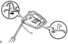
(c) Using a screwdriver wrapped with protective tape, disengage the 4 claws and disconnect the No. 1 room light assembly as shown in the illustration.
