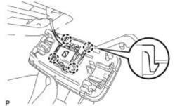
(d) Using a screwdriver, disengage the 4 claws and disconnect the room light switch base from the No. 1 room light assembly.
